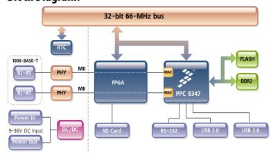
The Core module also provides provides the 8347 series PowerPC CPU, two USB 2.0 controller ports, indicator lights, timing/trigger interface, configuration ports and internal power supply. It's the brains of the Cube and controls the unit's operations including the interface with the host Controller (and other Cubes) and supervising the activity of the I/O Layers.
